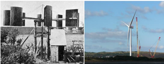
Figure 1: Blyth's 1887 turbine (left) compared to a modern-day Siemens SWT-6.0-154 (right). With a rotor diameter of 154 metres, the Siemens turbine is around 50 times bigger than Blyth's. (Siemens, 2015; Wikipedia).
